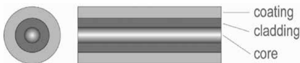
Figure 3: Optical Fiber Construction
